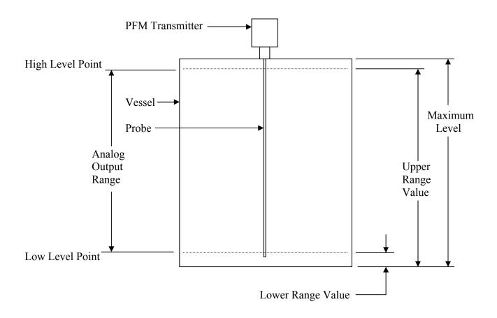
Determine the Maximum Level. This is the highest point that can possibly be measured. This is usually, but not always, the same as the tank height. Fill in the value below.
